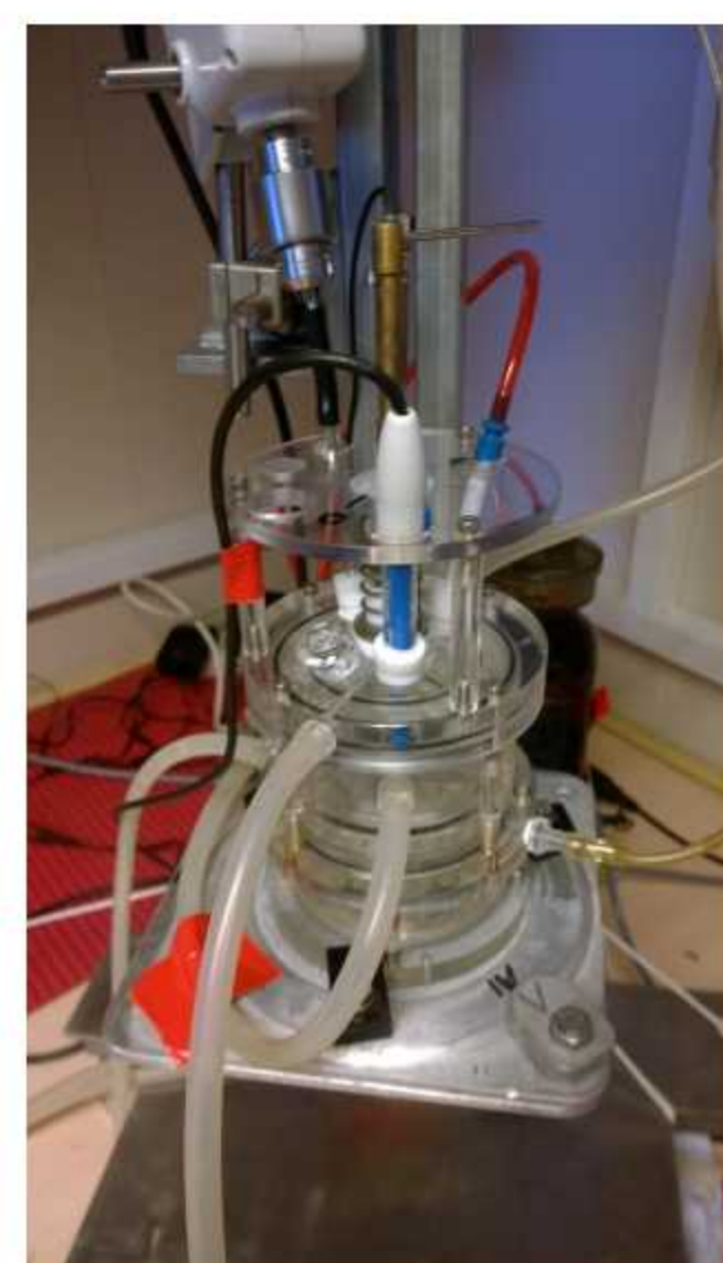
Figure 2 – Closed cell titration system for the determination of total alkalinity
