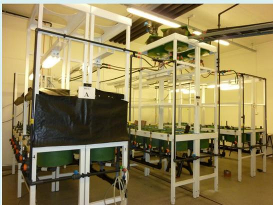
The Biolab consists of 3 rigs each containing 12 tanks with individual water supply.
